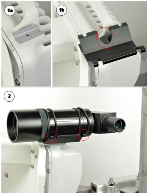
Figure 98: Attaching the telescope
