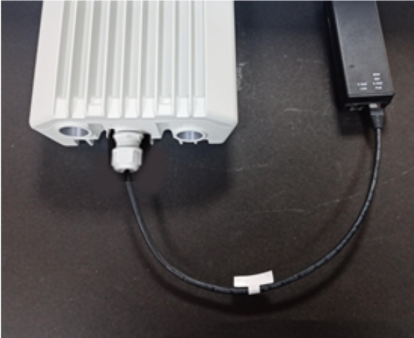
Figure 125: Connecting the power injector to ODU drop cable
