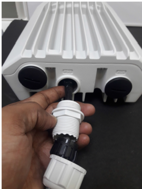
Figure 117: Removing the latch of the RJ45 plug
