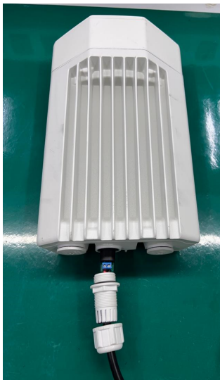
Figure 122: Connecting the input side of AC/DC PSU
