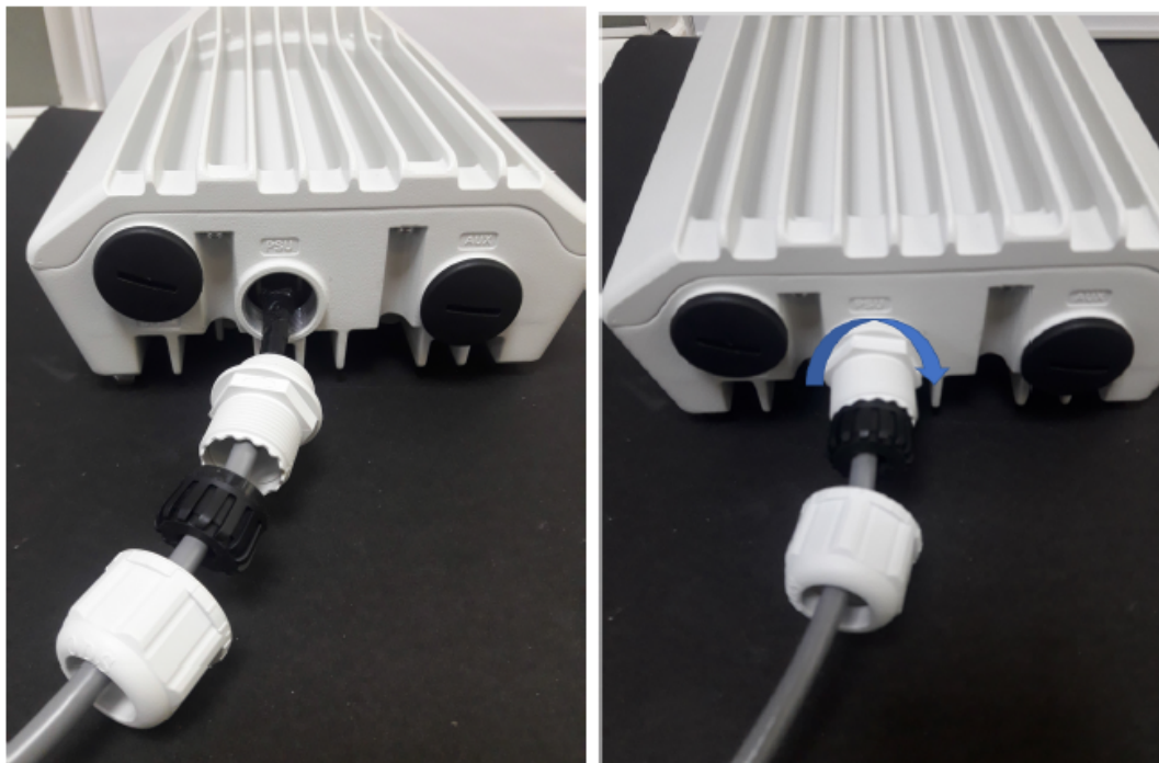
Figure 113: Connecting the RJ45 plug
