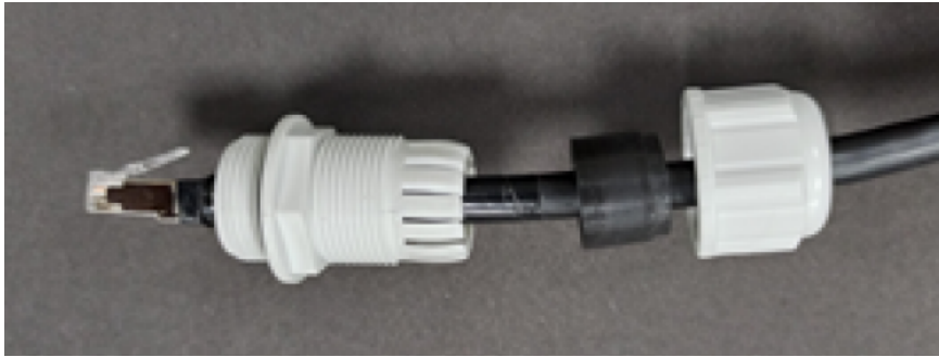
Figure 112: Fixing the gland nut
