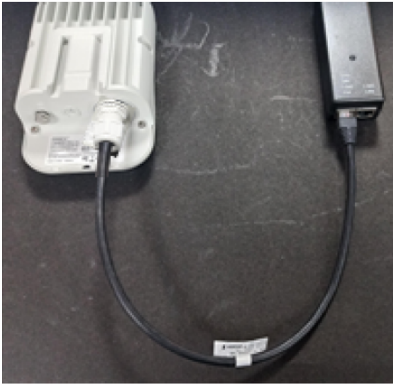
Figure 134: Connecting the V1000 Power injector
