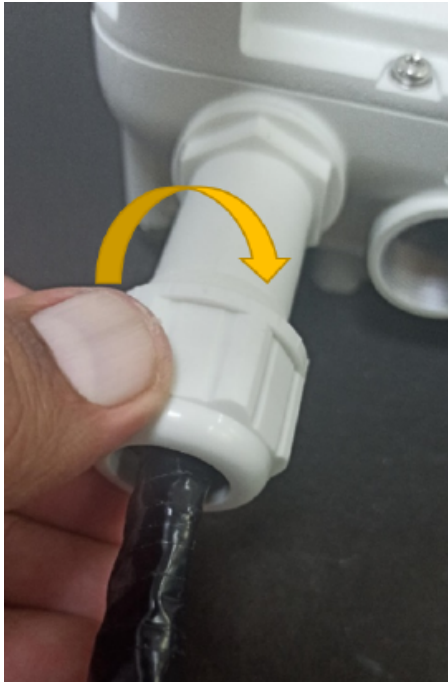
Figure 147: Fitting the gland nut
