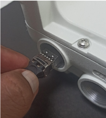
Figure 143: Rotating the latch
