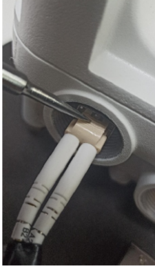
Figure 150: Pulling the bale clasp (latch)
