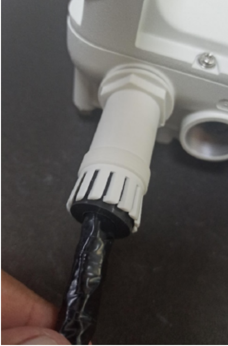
Figure 146: Fitting the gland body
