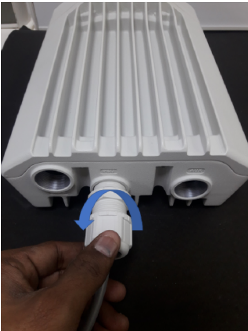
Figure 115: Removing the cable clamp
