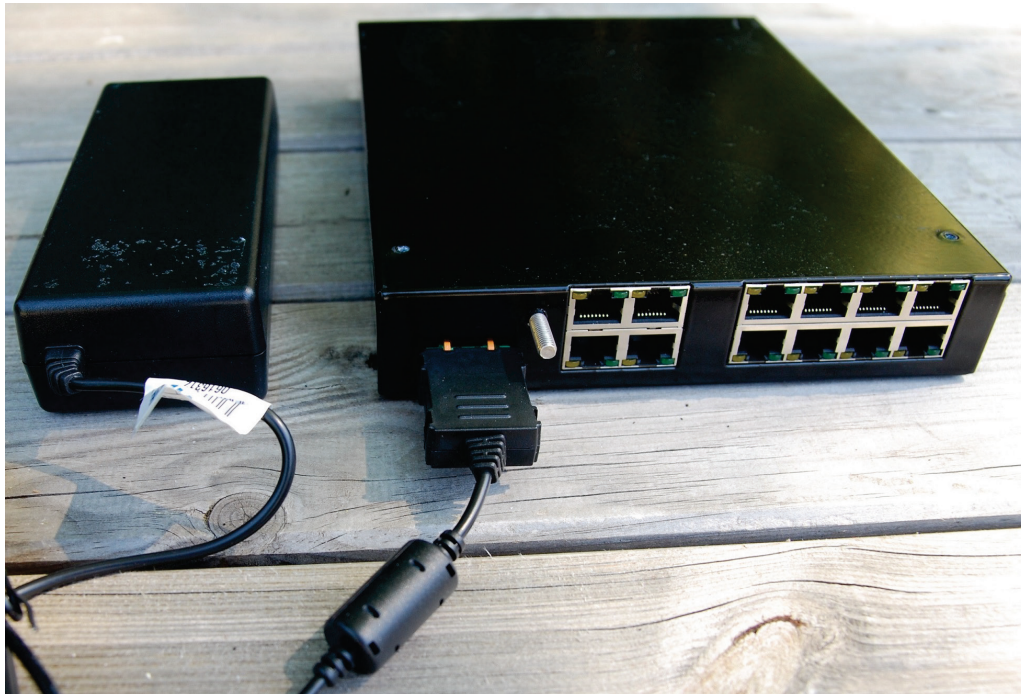
Figure 118 NIDU powered by the PTP 800 AC-DC Power Supply Converter
